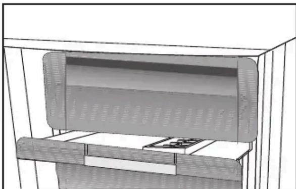
When deep-freezing hot food, the cooling compressor will work until the food is completely frozen. This can temporarily cause excessive cooling of the refrigeration compartment.
